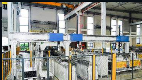
Automatic Landing Door Production Line
